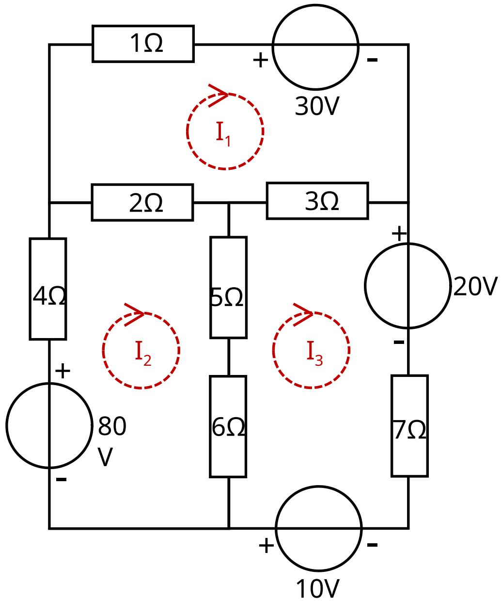
$$\begin{aligned} -30 &= (1+3+2) I_1 + -2 I_2 + -3 I_3 \\ 80 &= -2 I_1 + (2+5+6+4) I_2 + (-5-6) I_3 \\ -20 + 10 &= -3 I_1 + (-6-5) I_2 + (3+7+6+5) I_3 \end{aligned}$$
